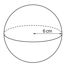
[The volume *V* of a sphere with radius *r* is  $V = \frac{4}{3}\pi r^3$ .]
